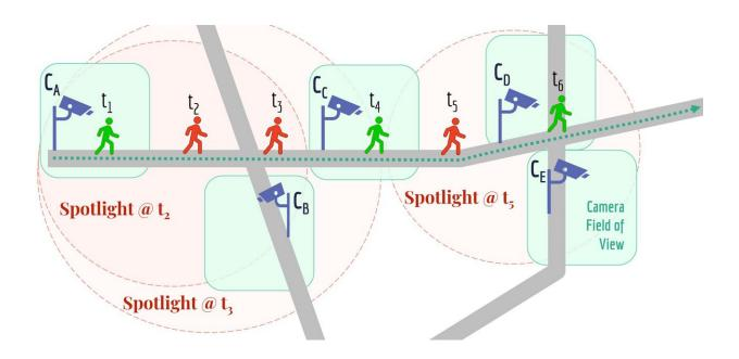
The spotlight algorithm narrows the search space for analysing video feeds if the missing person is found within a camera's field of view. It gradually expands the set of video feeds analysed when the person falls in a blindspot between cameras. This intelligence helps reduce the computation required for analysing videos from thousands of cameras while not sacrificing accuracy. Credit: Yogesh Simmhan
