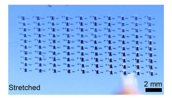
A closeup view of the design, which allows electronics to stretch without compromising data. Credit: Photo courtesy of Wang Group
