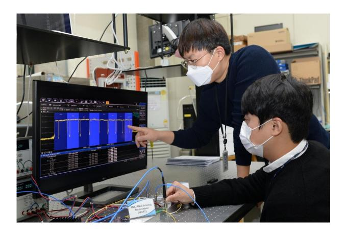
Researchers from ETRI are verifying the 5G indoor optical repeater's performance. Credit: Electronics and Telecommunications Research Institute(ETRI)
