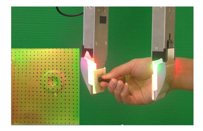
The tactile sensor used by the researchers. Credit: Bauza et al.
