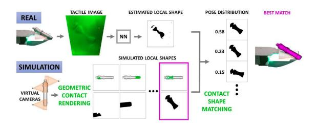
The researchers' approach helps robots localize objects through tactile sensing without requiring previous contact. (Bottom row) By developing a method to simulate contact as depth images, we can learn to match a pre-computed set of contacts against a real tactile observation (Top row) to estimate the current object pose. Credit: Bauza et al.
