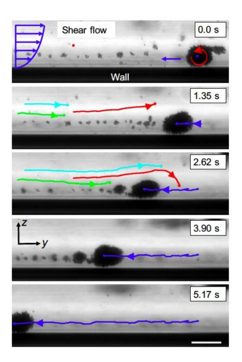
Image sequences demonstrate the rheotaxis of a microswarm rolling along the wall of the capillary (tracked in blue) in a combined acoustic and magnetic field. The streamlines of the oppositely directed flow are shown by cyan, green and red trajectories. Image 1: Credit: Ahmed et al.
