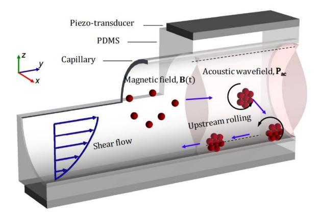
In a bioinspired system, superparamagnetic particles injected into the capillary self-assemble into a spinning microswarm due to the dipole–dipole interaction of a rotating magnetic field. The microswarm was shown to be marginalized towards the wall due to the presence of acoustic pressure nodes (marked as dashed black lines). Image 1: Credit: Ahmed et al.
