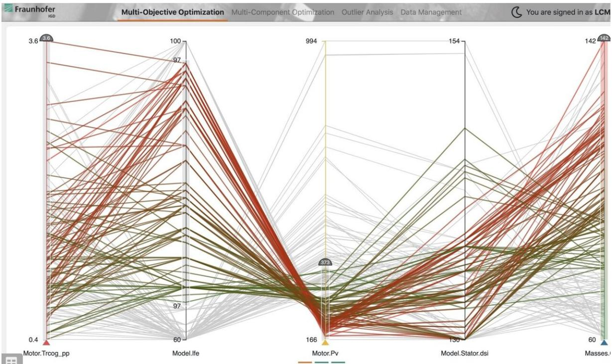
The visualization software displays hundreds of design alternatives as polylines. Typically, up to ten optimization criteria are observed at the same time. Credit: Fraunhofer IGD
