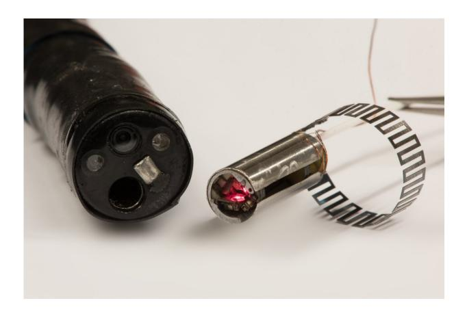
The microrobotic laser-steering end-effector (on the right) can be used as a fitted add-on accessory for existing endoscopic systems (on the left) for use in minimally invasive surgery. Credit: Wyss Institute at Harvard University
