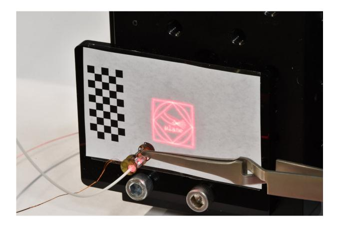
A long-exposure photograph shows the type of complex control that the lasersteering tool can perform. The image shows the laser-steering tool with the label "µlase" as shorthand for "Microlaser". Credit: Peter York/Harvard University
