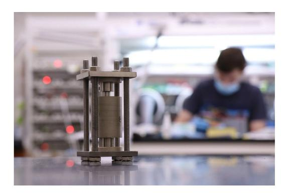
Solid-state batteries are charged and discharged in custom-made hardware designed at Georgia Tech. A smaller, modified version of the cell shown here was used to image these materials during cycling. Credit: Matthew McDowell, Georgia Tech
