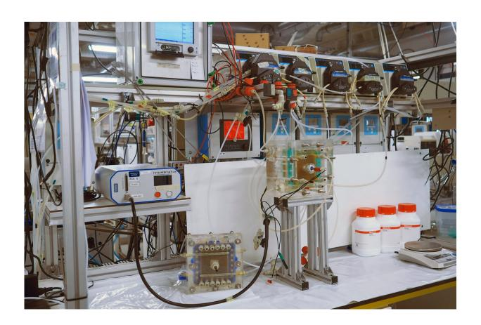
Lab-scale setup for capturing CO2 from seawater. Through the transparent module in the center, where green square seals and brown membranes are visible, (artificial) seawater containing CO2 flows, and the pH is successively lowered and raised, allowing the CO2 to be separated. Surrounding this module are pumps, regulating valves, pH meters, and a power source to keep this process going and to accurately monitor it. Credit: TU Delft/Rose Sharifian
