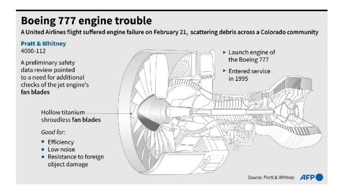
Factfile on the Pratt & Whitney 4000-112 engine used by Boeing 777 aircraft.
