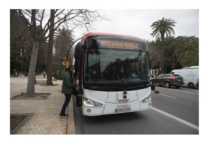
The electric-powered vehicle operates autonomously, but a driver still needs to sit behind the wheel as Spanish law doesn't allow self-driven vehicles yet
