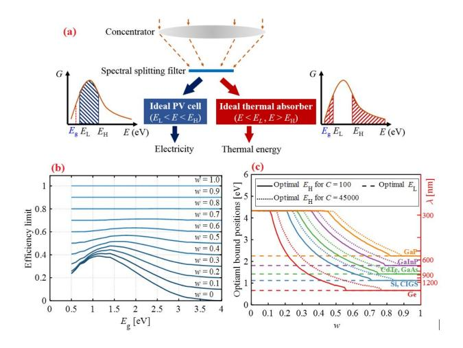
(a) Physical model of an ideal concentrating SSPVT collector. (b) Limit of total efficiency for different PV cells with different bandgap energies in different applications. (c) Optimal spectral-splitting filters for common PV cell materials. Credit: Gan Huang, Kai Wang and Christos N. Markides.
