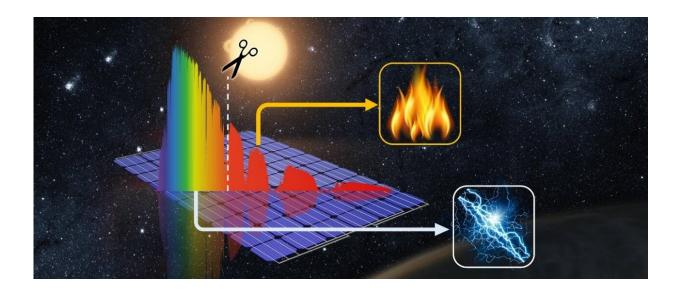
The solar spectrum is separated by an optical filter, and only part of the spectrum is sent to the PV cells for electricity generation. The rest of the spectrum, which cannot be utilized by the solar cells, is directed to a thermal absorber to generate thermal energy. Credit: Gan Huang, Kai Wang and Christos N. Markides.
