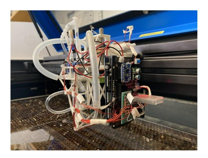
The MIT CSAIL team's LaserFactory system can manufacture functional, custom-made devices and robots, without human intervention, potentially enabling rapid prototyping of items like wearables, robots, and printed electronics. Credit: Massachusetts Institute of Technology
