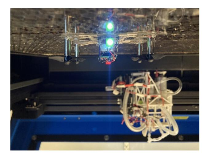
LaserFactory (in background) can fabricate fully functional drones like this quadcopter. Credit: Massachusetts Institute of Technology
