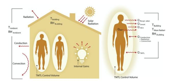
Schematic of thermal interactions with the environment and energy transfers that are needed for the theoretical minimum thermal load (TMTL) calculation. Credit: Julia Laser and Josh Bauer, NREL
