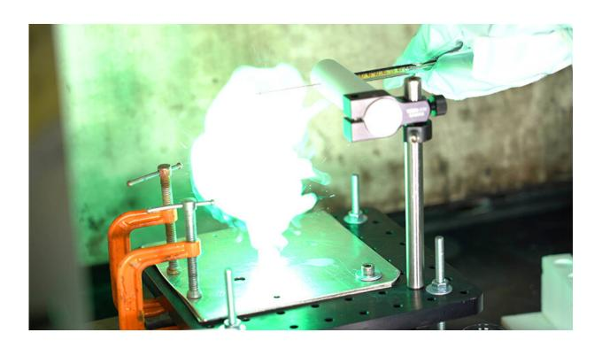
Ammonia borane is a hypergolic propellant that releases a brilliant green flash when exposed to an oxidizer. Purdue researchers are developing ammonia borane as a safer alternative to current hypergolic fuels. Credit: Purdue University photo/Jared Pike
