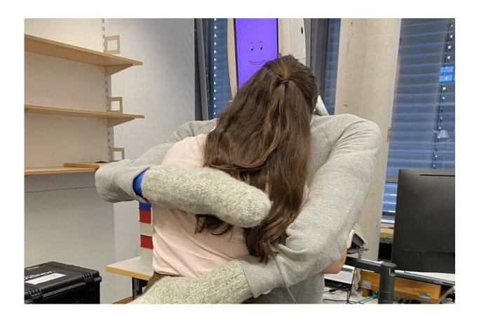
HuggieBot 2.0 hugging a user. Haptic sizing enables the robot to embrace the user securely and safely and redundant sensors let it know when the user is ready for the hug to end. Credit: Block et al.
