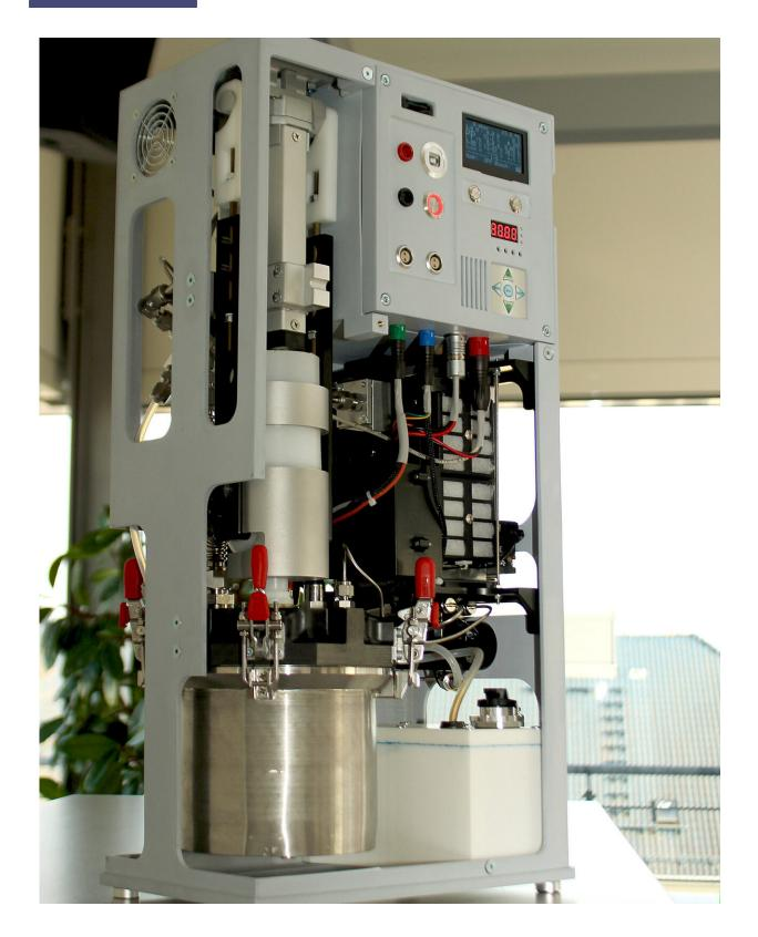
TRL 5 demonstrator of a power generator with a POWERPASTE cartridge and a 100 watt PEM fuel cell. Credit: Fraunhofer-Gesellschaft
