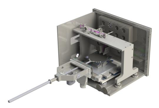
Interference chamber for full-wafer experiments. Credit: IMEC
