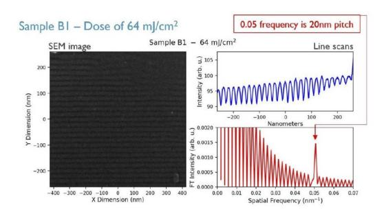
(Left) Cross-section SEM image of a 20nm L/S pattern imaged an Inpria metal-oxide resist, exposed in a Lloyd's mirror interference setup at a dose of 64mJ/cm2 and interference angle 20°. (Right) Fourier transform analysis where 0.05=20nm pitch. Credit: IMEC
