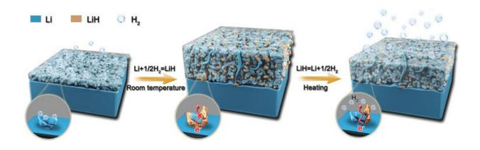
The temperature sensitive equilibrium governing the formation and decomposition process of LiH at Li anode. Credit: Xu Gaojie
