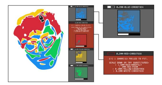
Fabricaide provides live feedback on laser-cut designs, such as warnings about whether the materials will fit on the sheets to be cut. Credit: Massachusetts Institute of Technology
