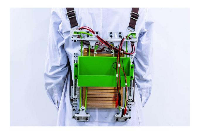
A prototype backpack harvests energy from walking to power small electronics, and it makes loads feel lighter. Credit: Adapted from *ACS Nano* 2021, DOI: 10.1021/acsnano.0c07498
