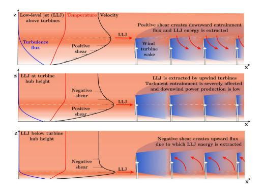
The amount of energy extracted from low-level jet flow is severely impacted by whether the wind turbines are operating below, at the same height as, or above the low-level jet. Credit: Srinidhi N. Gadde and Richard J.A.M. Stevens
