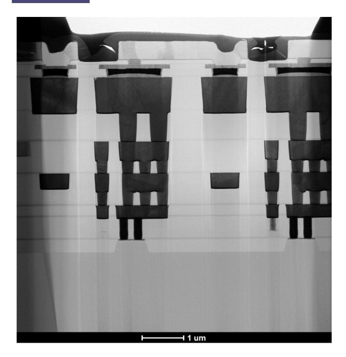
A cross-section of one of the wafers that the researchers used in their experiments. All of the black rectangles in-between the transistor (bottom) and the memristors (top) are four metal layers. In the researchers' chip, these layers were used to connect-up the circuits composed of CMOS transistors and memristors. At the bottom, one can make out the drain and source of a transistor. Credit: Dalgaty et al.
