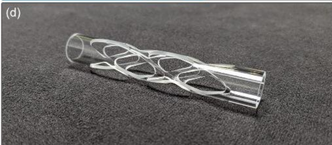
Cutting of glass tubes with complex inner and outer contours. Credit: Daniel Flamm et al.
