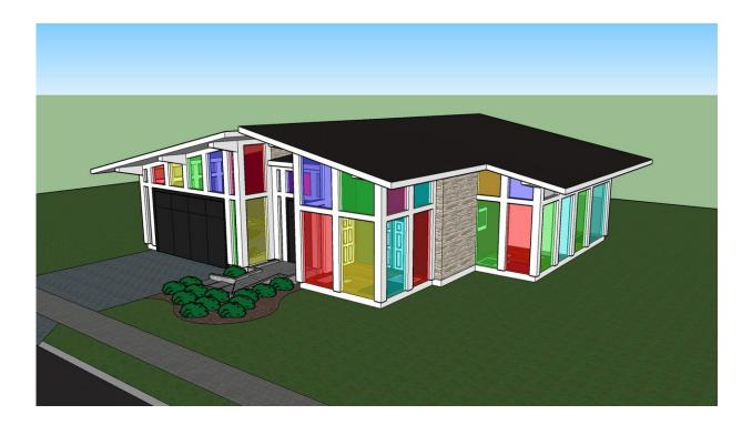
A concept for a house using windowpanes designed by Rice University engineers to redirect light from inside and out to edge-band solar cells. Credit: Yilin Li
