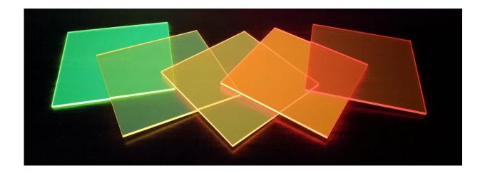
Rice University engineers designed and built windowpanes that redirect sunlight or illumination from indoors to edge-band solar cells. The central layer is a conjugated polymer that serves as a waveguide. Credit: Yilin Li
