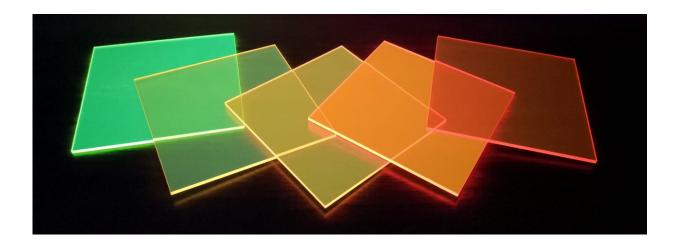
Rice University engineers designed and built windowpanes that redirect sunlight or illumination from indoors to edge-band solar cells. The central layer is a conjugated polymer that serves as a waveguide. Credit: Yilin Li
