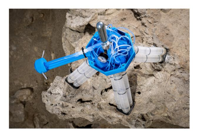
The robot relies on a series of valves that open and close in a specific sequence to walk. Credit: University of California San Diego
