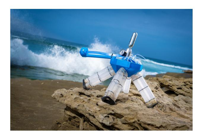
Engineers at the University of California San Diego have created a four-legged soft robot that doesn't need any electronics to work. The robot only needs a constant source of pressurized air for all its functions, including its controls and locomotion systems. Credit: University of California San Diego
