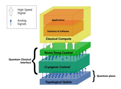
Figure 1: Quantum stack diagram. Topological qubits sit at the bottom of the stack in the quantum plane along with other electronics needed to help with the processing of information from raw qubits. The Gooseberry chip sits very near the qubits, while Alta is positioned at the bottom of the "Classical Compute" portion of the stack, where it is in communication with both Gooseberry and components higher up the stack. Credit: Microsoft
