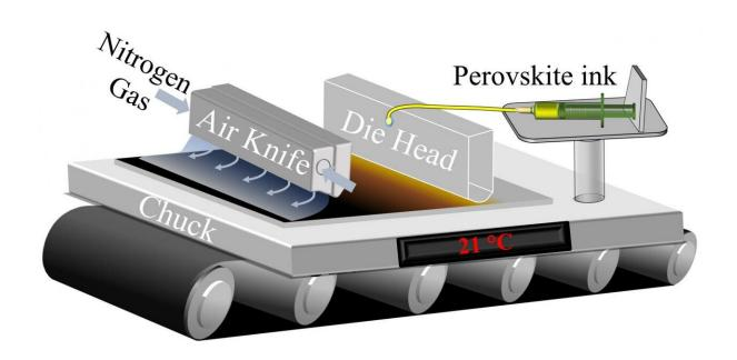
The liquid solution of perovskite precursor, solvent, and additive flows from a slit-shaped nozzle onto the glass substrate being conveyed below. Credit: HZB/Jinzhao Li
