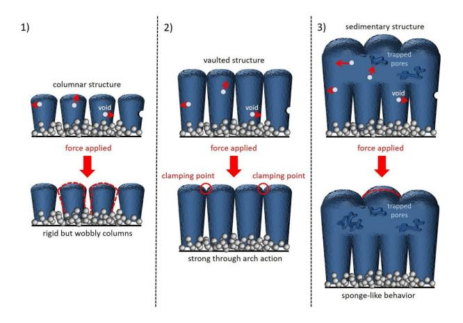
In the first stage, the silicon film exists as a rigid but wobbly columnar structure. In the second stage, the columns touch at the top, forming a vaulted structure, which is strong due to arch action. In the third stage, further deposition of silicon atoms results in a sponge-like structure. The red dashed lines show how the silicon deforms as a force is applied. Credit: Dr. Panagiotis Grammatikopoulos, OIST Nanoparticles by Design Unit and Particle Technology Laboratory, ETH Zürich
