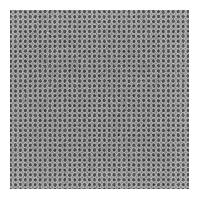
28nm contact holes obtained on a 0.33NA NXE:3400 full field scanner, after developing. Credit: IMEC
