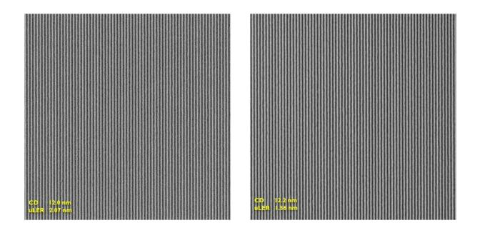
24nm pitch line/spaces obtained on a 0.33NA NXE:3400B full field scanner, (left) after developing and (right) after etching on target critical dimension (CD) (uLER = unbiased line-edge roughness). Credit: IMEC
