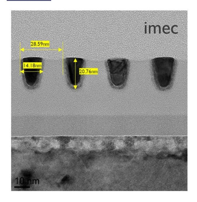
28nm pitch single-exposure patterning using Inpria's MOx process on a 0.33NA EUV full field scanner after Ru metallization. Credit: IMEC
