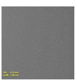
24nm pitch line/spaces obtained on a 0.33NA NXE:3400B full field scanner, (left) after developing and (right) after etching on target critical dimension (CD) (uLER = unbiased line-edge roughness). Credit: IMEC
