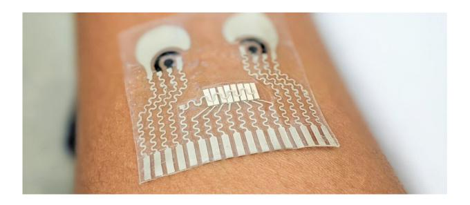
This soft, stretchy patch can monitor the wearer's blood pressure and biochemical levels at the same time. Credit: Wang lab/UC San Diego
