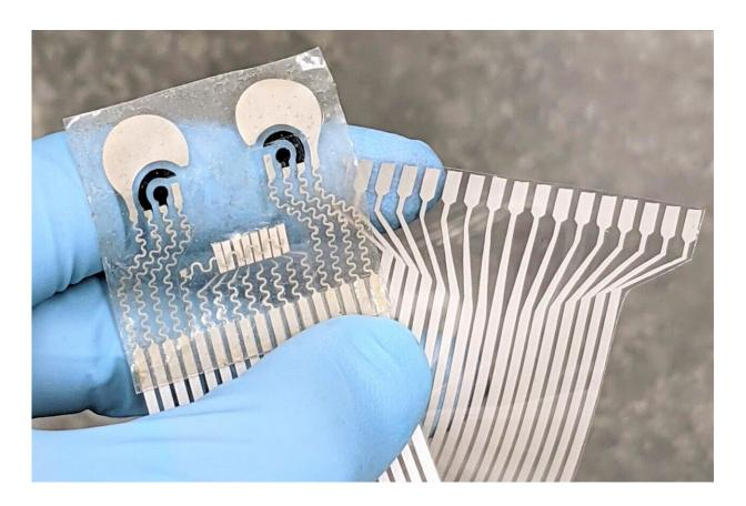
The current prototype of the patch needs to be wired to a benchtop machine and power source. Credit: UC San Diego
