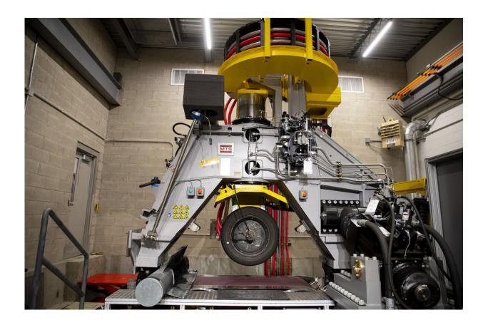
The MTS CT Plus Flat Trac measures forces on a moving tire. Sandia National Laboratories has worked with Goodyear to develop a Virtual Flat Trac. Credit: Smithers
