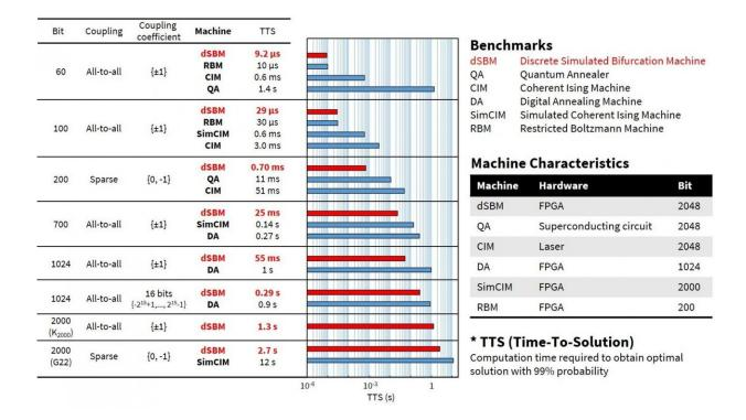
dSBM benchmarked against other machines for computation times to obtain optimal solutions for various problems. Credit: Toshiba Corporation
