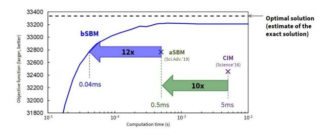
The bSBM is approximately 10x faster than the aSBM in solving a 2000-bit problem. Credit: Toshiba Corporation
