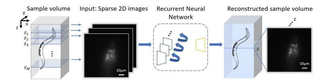
Recurrent neural network-based 3D fluorescence image reconstruction framework. Credit: Ozcan Lab, UCLA
