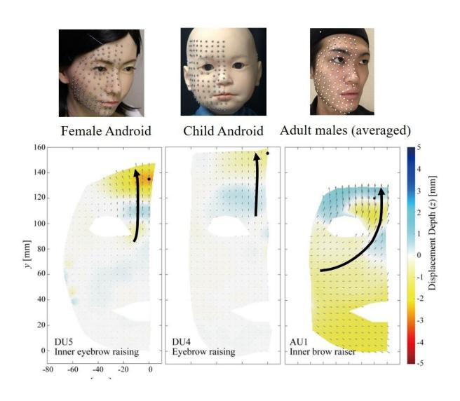
Example of the facial flow lines when two androids (left and middle) and adult males (right) lifted their inner eyebrow. Credit: Ishihara, Iwanaga, and Asada, Comparison between the Facial Flow Lines of Androids and Humans, *Frontiers*
