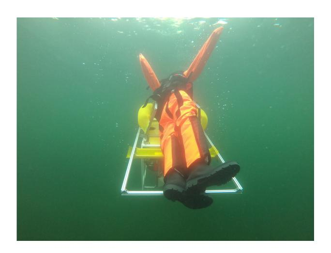
During testing at the Hufeisensee lake, the dummy did not slip out of the securing mechanism as it was taken to the surface. Credit: S.Thomas (Wasserwacht Halle)
