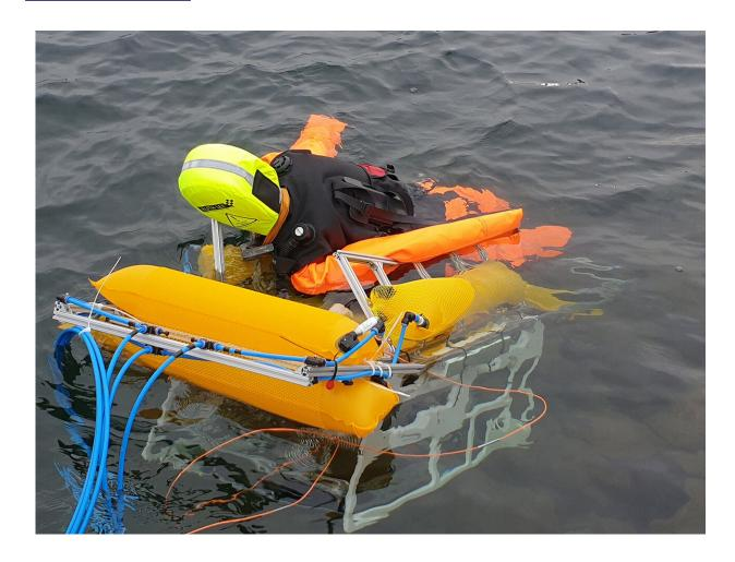
The aquatic robot transports the dummy to shore via the shortest route.© Fraunhofer IOSB-AST
