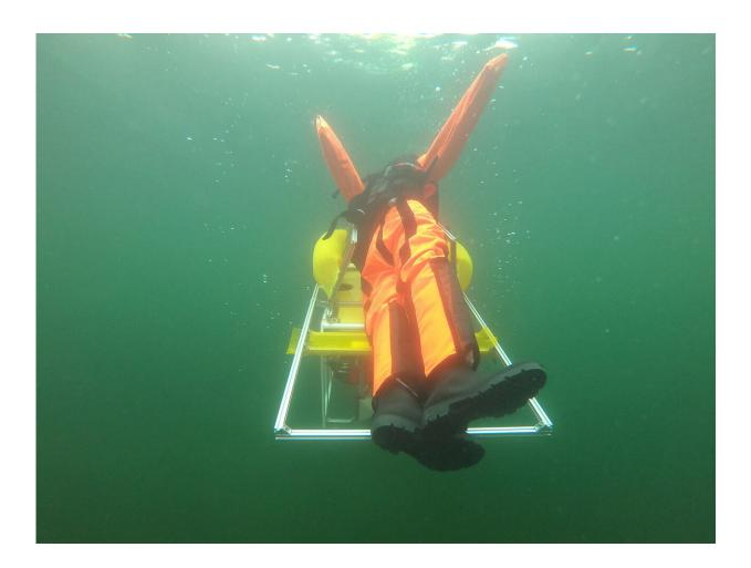
During testing at the Hufeisensee lake, the dummy did not slip out of the securing mechanism as it was taken to the surface. Credit: S.Thomas (Wasserwacht Halle)
