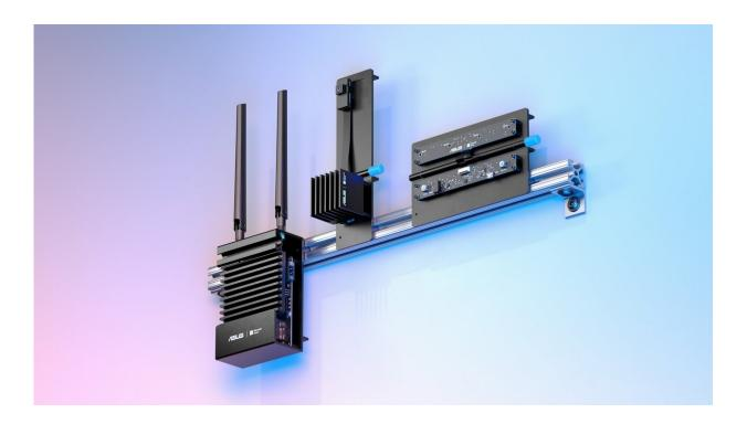
Azure Percept devices, including Trust Platform Module, Azure Percept Vision and Azure Percept Audio. Credit: Microsoft
