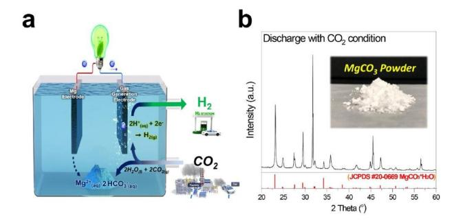
(a) Schematic illustration of MF Mg-CO2 battery. (b) The XRD profile of the precipitated white solid after discharge process in CO2 sat'd condition and N2 sat'd condition. Credit: Ulsan National Institute of Science and Technology
