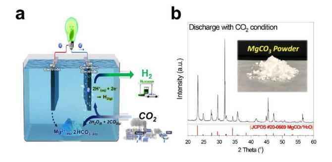
(a) Schematic illustration of MF Mg-CO2 battery. (b) The XRD profile of the precipitated white solid after discharge process in CO2 sat'd condition and N2 sat'd condition. Credit: Ulsan National Institute of Science and Technology
