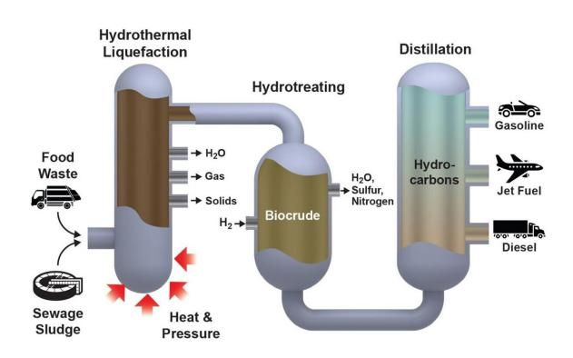
Wet wastes from sewage treatment and discarded food can provide the raw materials for an innovative process called hydrothermal liquefaction, which converts and concentrates carbon-containing molecules into a liquid biocrude. This biocrude then undergoes a hydrotreating process to produce bio-derived fuels for transportation. Credit: Michael Perkins/Pacific Northwest National Laboratory
