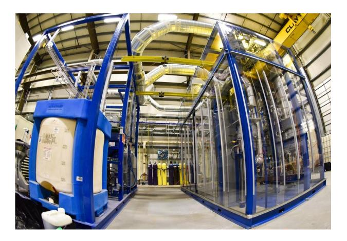
This reactor turns wet waste into biocrude, which in turn feeds a refining step that turns biocrude into fuels for transportation. Credit: Andrea Starr/Pacific Northwest National Laboratory
