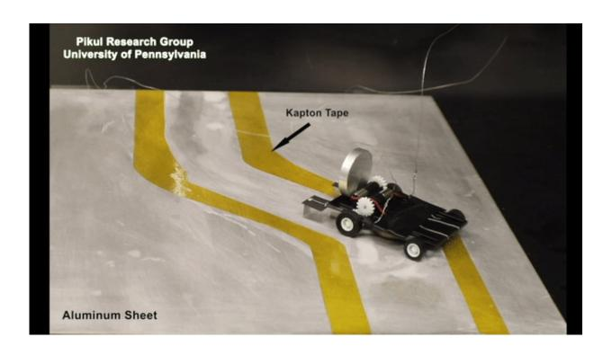
The "metal-eating" robot can follow a metal path without using a computer or needing a battery. By wiring the power-supplying units to the wheels on the opposite side, the robot autonomously navigates away from the tape and towards aluminum surfaces. Credit: University of Pennsylvania
