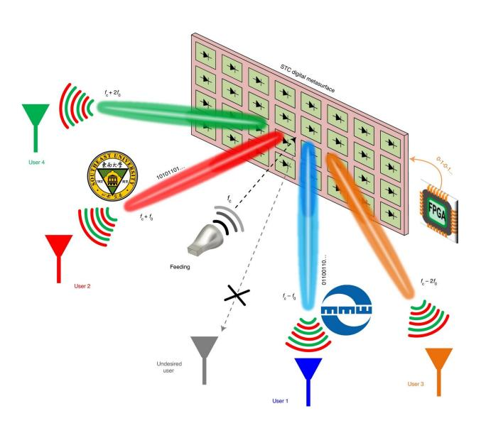
By applying different control voltages from the FPGA to PIN diodes, the reflection phases of metasurface elements are periodically switched according to
