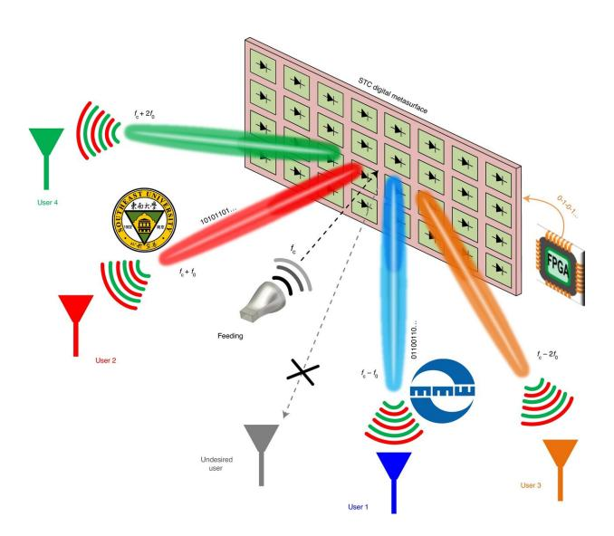
By applying different control voltages from the FPGA to PIN diodes, the reflection phases of metasurface elements are periodically switched according to
