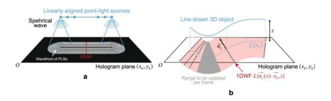
Overview of the CG-line method. (a) Principle of obtaining 1DWF. (b) Method to create CGH using the CG-line method in the proposed system. Credit: *Scientific Reports* (2021). DOI: 10.1038/s41598-020-78902-1
