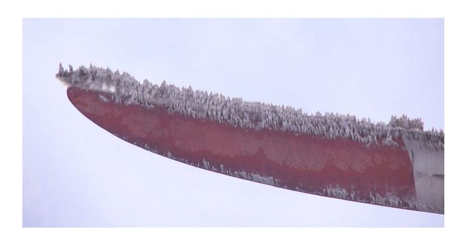
This drone photo from a field study of icing on wind turbines shows how ice accumulated at the tip of a turbine blade during a winter storm. Credit: Hui Hu/Iowa State University
