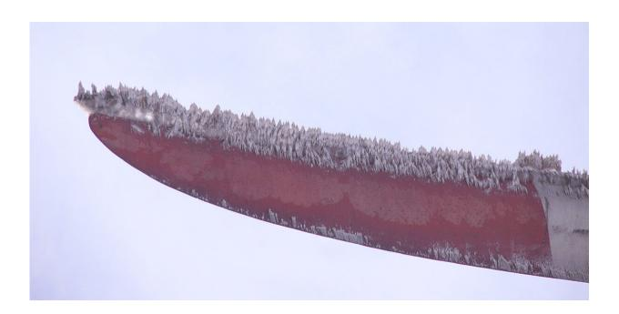
This drone photo from a field study of icing on wind turbines shows how ice accumulated at the tip of a turbine blade during a winter storm. Credit: Hui Hu/Iowa State University
