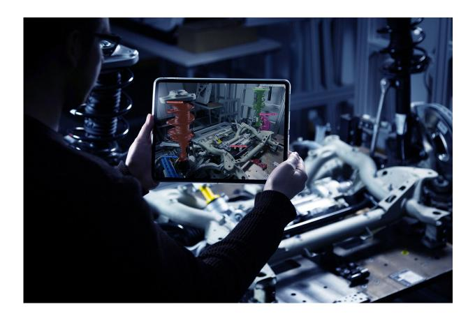
MARQUIS software recognizes both the component itself, and also any discrepancies from the target dimensions. Credit: Fraunhofer-Gesellschaft
