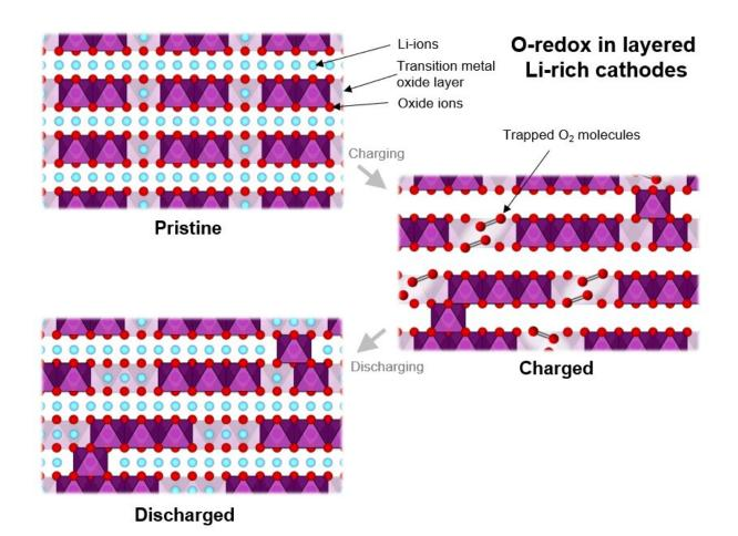
The structure of a Li-rich cathode in a pristine, charged and discharged state showing how molecular O2 takes part in the energy storage mechanism of an Oredox material. Credit: Dr Robert House, University of Oxford
