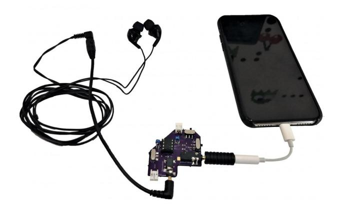
"Dumb" headphones can be plugged into a HeadFi device that connects to a cellphone, turning them into intelligent headphones. Engineers are working on a smaller version of the device. Credit: Siddharth Rupavatharam
