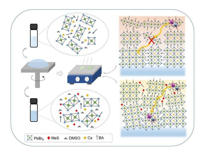
Effects of MeS on phase distribution of perovskite films. The yellow path indicates the exciton energy transfer between nanosheets of different thicknesses. Credit: Lingmei Kong et al.
