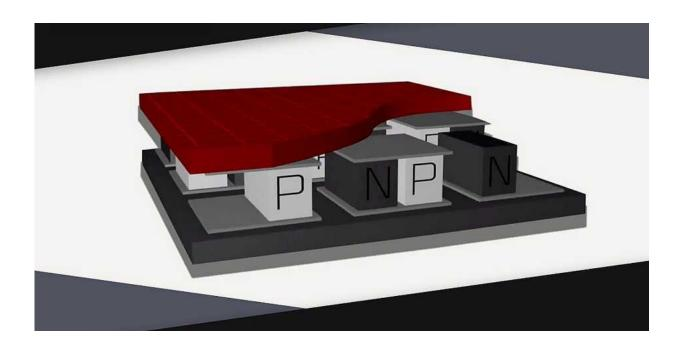
The core of Mithras technology, the thermoelectric foil, consists of a sequence of semiconductor elements connected with conductive metal. At the top (in red) is the thermal interface. Credit: Mithras Technology
