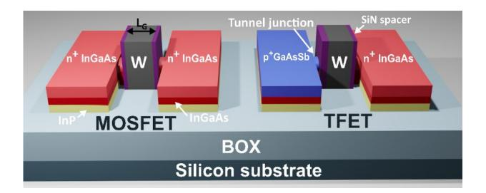
3D schematic representing the developed technology platform. The MOSFET (on the left) differs from the Tunnel FET (on the right) only in the use of different materials in the transistor source region. Credit: Convertino et al.
