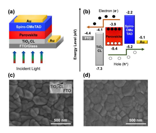
(a) The schematic diagram and (b) corresponding energy levels of the investigated single-junction planar perovskite solar cell. Top-view scanning electron microscopy (SEM) micrographs of (c) spray-pyrolysis deposited  $TiO_2$  compact layer (the inset shows the cross-sectional view of the  $TiO_2$ ), and (d) perovskite film deposited on  $TiO_2$ -CL/FTO substrate. The  $TiO_2$  precursor solution has a concentration of 0.35 M and a thickness of 70 nm. Credit: Kanazawa University
