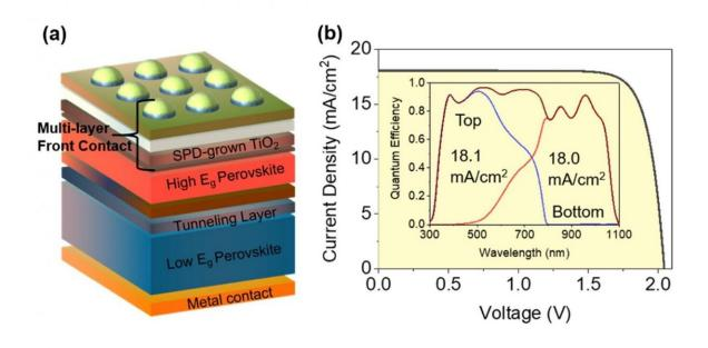
(a) Schematic diagram of the perovskite/perovskite tandem solar cell, and (b) current-voltage characteristic curves of the best-investigated perovskite/perovskite tandem solar cell. Inset shows quantum efficiency for top perovskite and bottom perovskite. Credit: Kanazawa University
